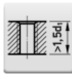
HOLE TYPE Through hole (thread length L > 1,5 \times d1 )
