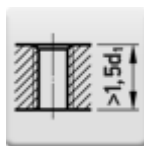
HOLE TYPE Through hole (thread length L > 1,5 \times d1 )
